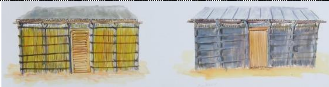
Fig. 6. Facade of an unplastered quincha house in Santa Rosa, and facade of a quincha house, with mud plaster, in Santa Rosa.
