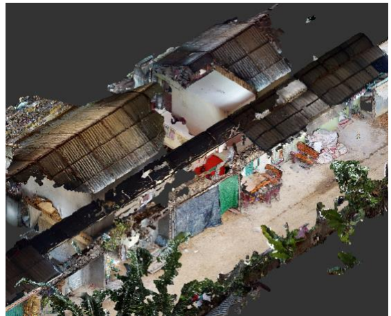
Fig. 8. Screenshot of point cloud model taken by matterport pro2 camera, showing kind of visual representation shared
