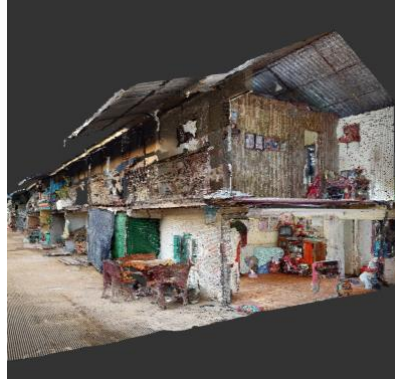
Fig. 5. Point Cloud model captured by Matterport pro2 camera and viewed in AutoDesk Recap
