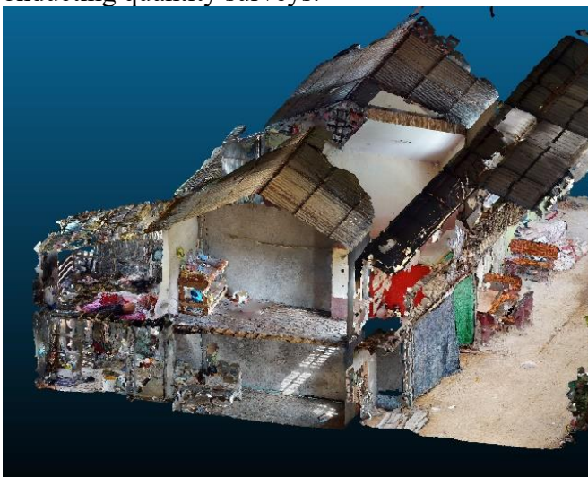
Fig. 9. Screenshot of sectional view of point cloud model on CloudCompare software
